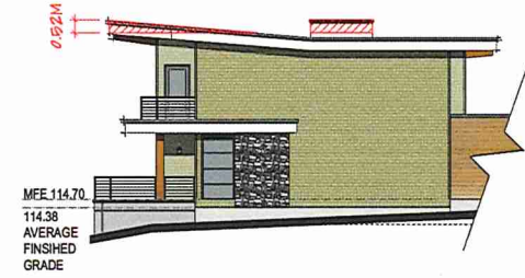
EAST ELEVATION UNIT 3
